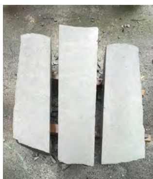
Basalt stone column sliced into three sections to make one of the two stone bridges.
